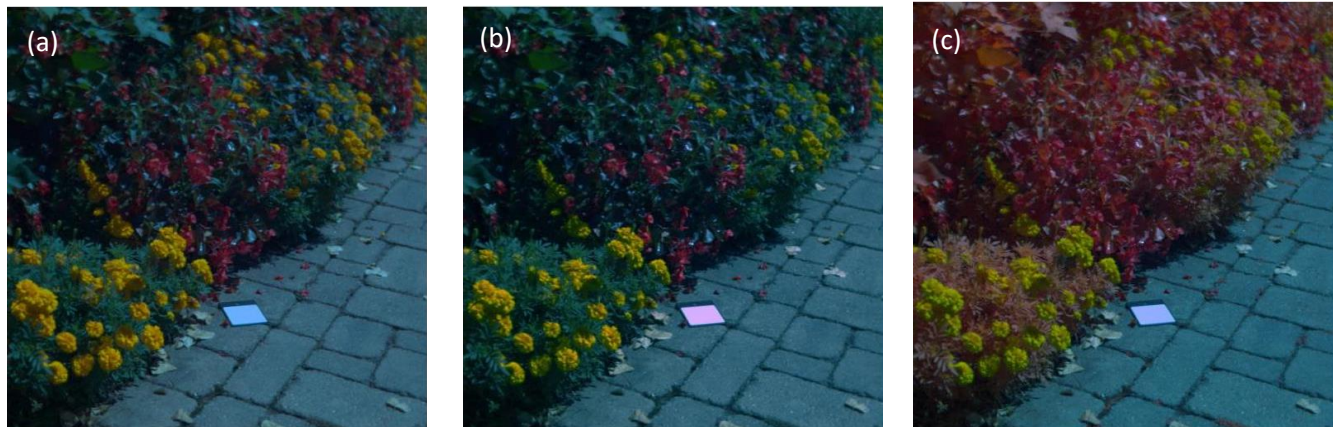
Fig 1. (a) True color image produced from the normalized reflectance spectrum. Replacing R with R' to produce a false color image where (b) \lambda_1 = 620 nm, \lambda_2 = 710 nm and (c) \lambda_1 = 770 nm, \lambda_2 = 810 nm.
